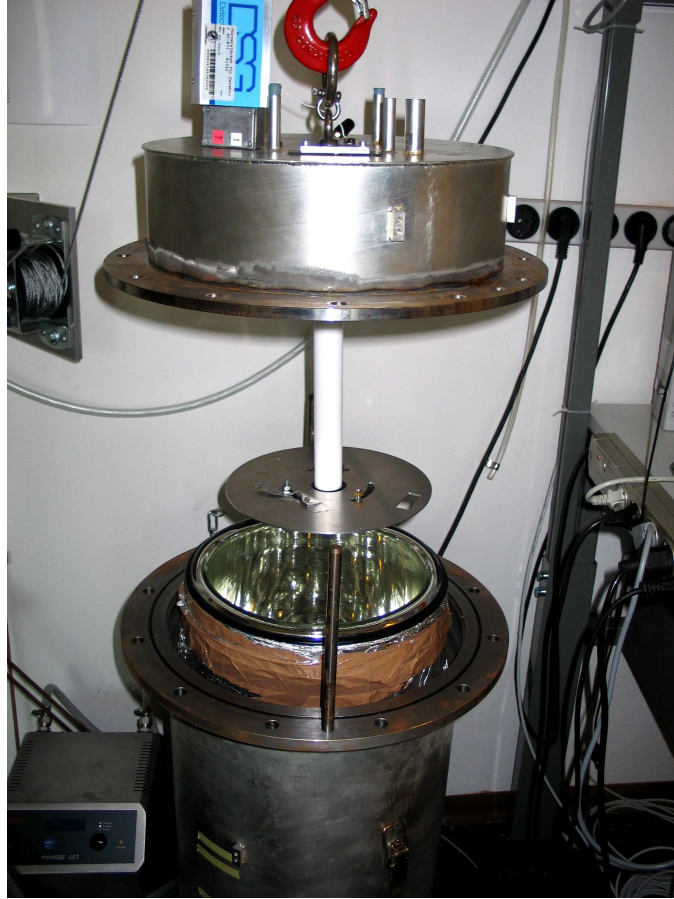
Figure 4.2: Test stand used for this experimental analysis. It is a small version of the GERDA set-up at LNGS in Italy. The detector is suspended into the liquid Argon dewar.
