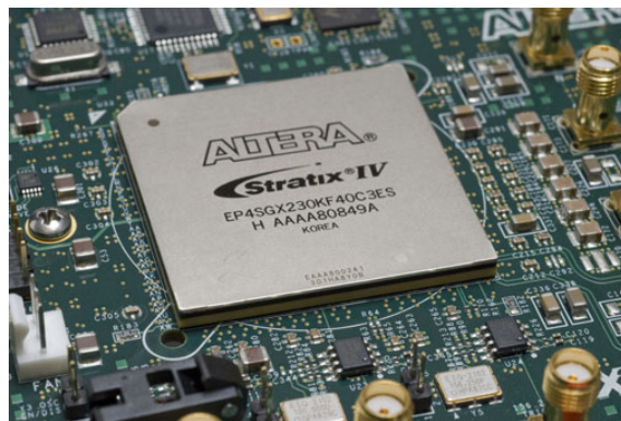
Figure 3.1: Picture of a modern Altera Stratix IV FPGA embedded in a development board.
